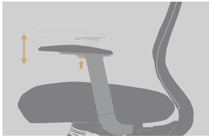
Armrest lifting adjustment 7, adjusting distance 80 mm
