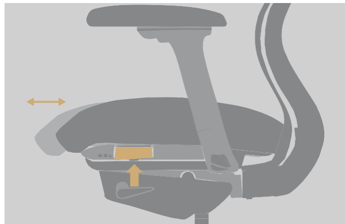
Seat depth adjustment 6, adjusting distance 50 mm
