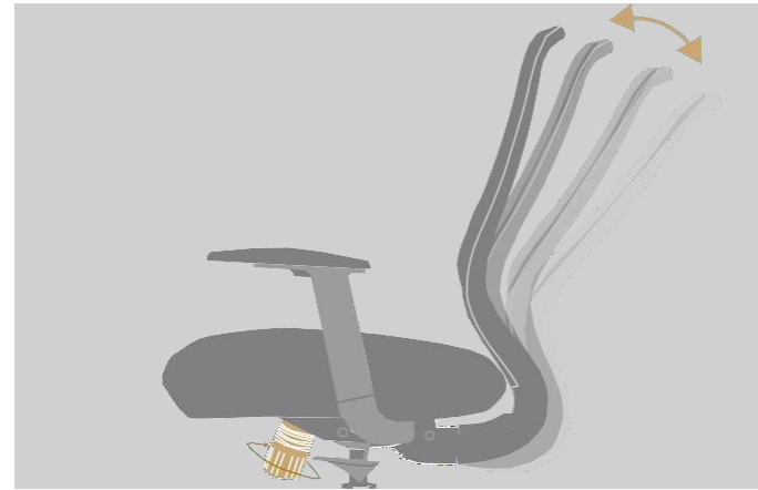
Tilt elastic adjustment gear, adjustment range 20 degrees
