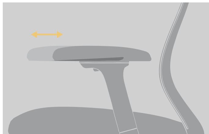
Back adjustment of handrail, adjusting distance 45mm
