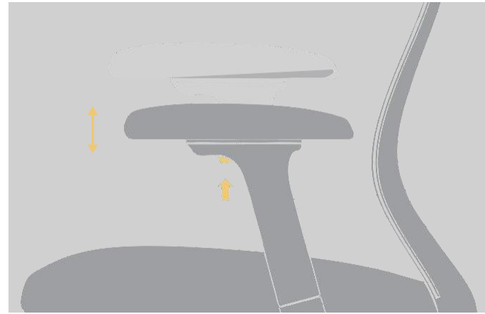
Armrest lifting adjustment 7, adjusting distance 80 mm
