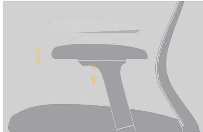
Armrest lifting adjustment 7, adjusting distance 80 mm
